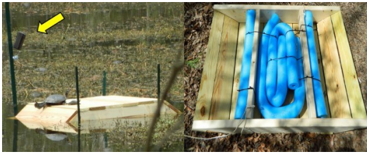
Figure 1: Artificial basking platforms deployed during this study showing 1 adult and 1 juvenile Trachemys scripta with arrow highlighting trail camera (left) and underside of platforms composed of several wood support frames and polyethylene foam attached with zip ties for increased floatation (right).
